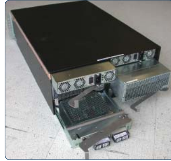
From the rear of the SANbox 9000 chassis module, customer replaceable CPU 1 , power supply and fan blades are accessible.
