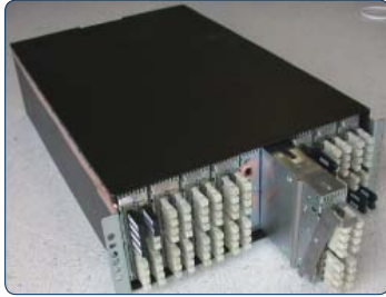
From the front of the SANbox 9000 chassis module, up to 8 customer serviceable I/O and SSP blades can be added or replaced non-disruptively without tools.
